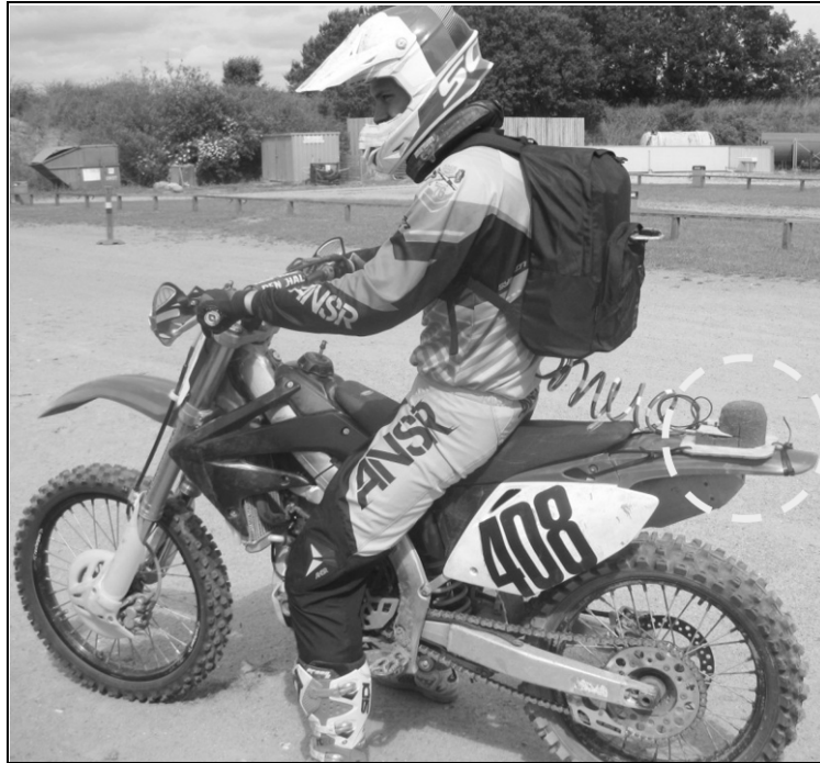
Figure 2 Motocross test driver equipped with rucksack on the back and the microphone mounted at the rear mudguard of the bike.
