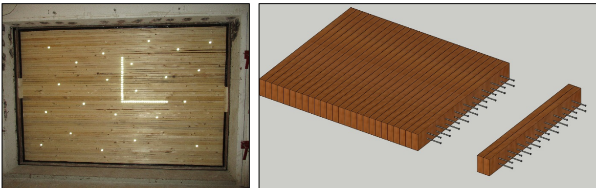
Figure 1: NLT installed in the laboratory and a schematic of the NLT construction. The bright spots in the photo are reflective tape which was used for the measurements of the surface velocity with the laser vibrometer.
